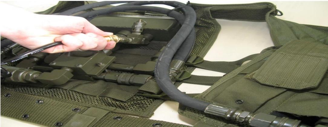
**Step 2:** While charging, keep the CO2 charging kit connected to the unit until the sound of pressurized air has stopped completely. Once the sounds of pressurizing air has stopped completely, then turn the handle on the CO2 tank counter-clockwise until the valve stops turning. This will close the cylinder, once it is closed remove the pressure line from the vest. The vest is now filled with paint and pressure and is ready to be deployed on a mission.
