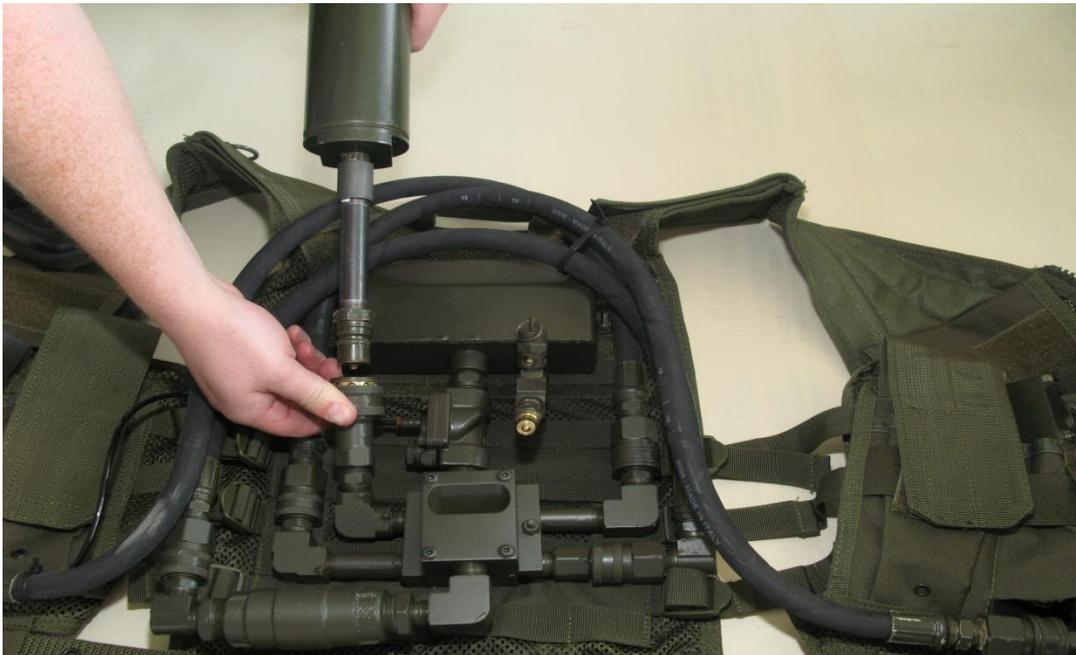
**Step 4:** Make sure the Injector Cylinder is firmly in place. Depress the cylinder by pushing the handle down until the handle stops. Once the stroke is complete, release the port release to remove the Injector from the filling port. You have now successfully energized the Suicide Vest with paint.
