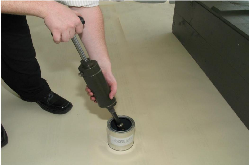
**Step 3:** With the Injector Cylinder full of paint, take it to the filling port on the back of the vest. Push the tip of the Injector Cylinder into the filling port, with your free hand pull the release on the vest down which should enable the Injector to “click” into place.
