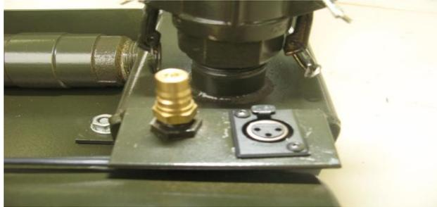
**Step 2:** Turn the knurled knob at the top of the liquid CO2 bottle on the Charging Kit clockwise until the sound of rushing gas is heard. "Wait" approximately 60 seconds or longer. Turn the knurled knob counterclockwise until the knob becomes loose.
